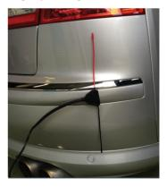
ALWAYS MOUNT THE ANTENNA VERTICALLY WITH THE RED COLOURED RADIAL POINTING UPWARD.
